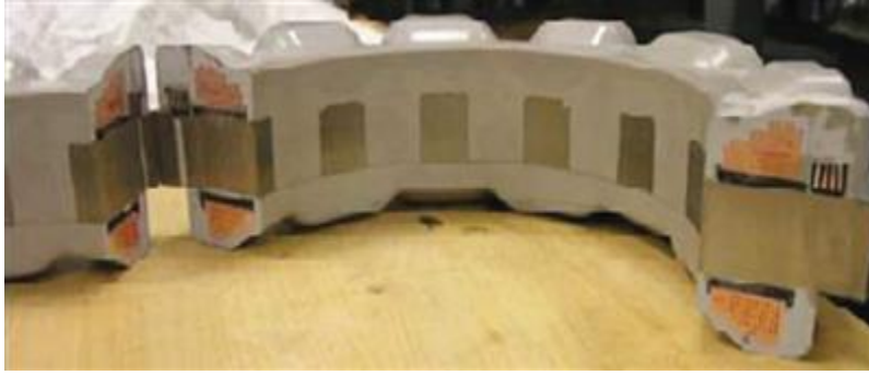
Figure 17.33 Cutout of the Prius 2010 FSCW-PM generator stator winding [101]
