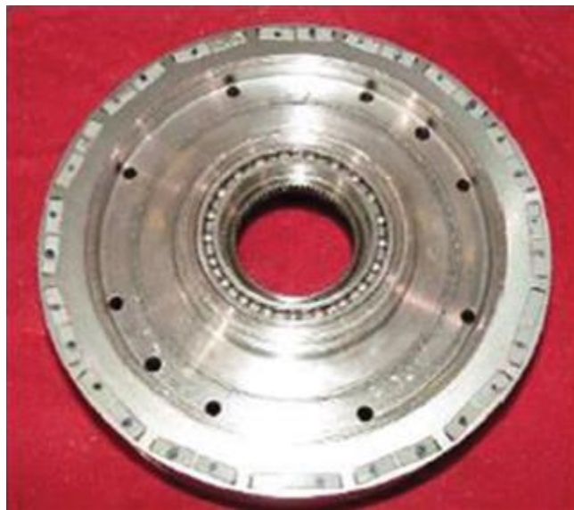
Figure 17.36 Machine A rotor with the end ring removed to show the magnet arrangement [102]
