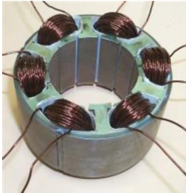
Figure 17.4 Example of concentrated windings around one tooth with an irregular distribution of slots
