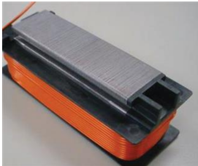
Figure 17.34 One-tooth assembly of the Voltec motor A [102]
